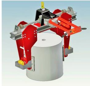
Roll tooling with push-off tool to transfer the roll to another shaft
